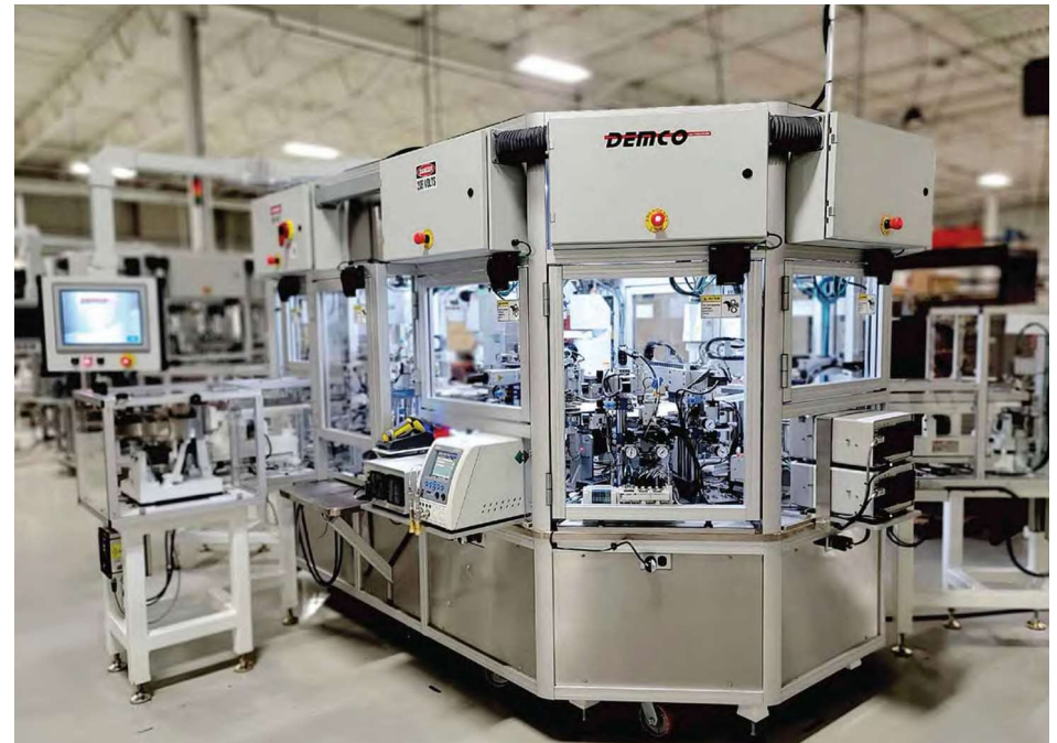
A pair of rotary indexing dials are used to assemble an actuation device for a surgical instrument. Photo courtesy Demco Automation.
